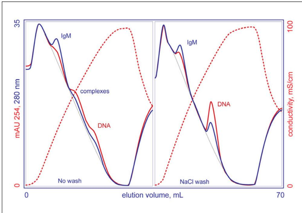
FIGURE 9. Comparison of HA profiles illustrating the ability of a pre-elution salt wash to promote dissociation of IgM-DNA complexes. The first profile illustrates phosphate-NaCl gradient elution without a previous wash. The second, a 2M NaCl wash applied before the same gradient.
