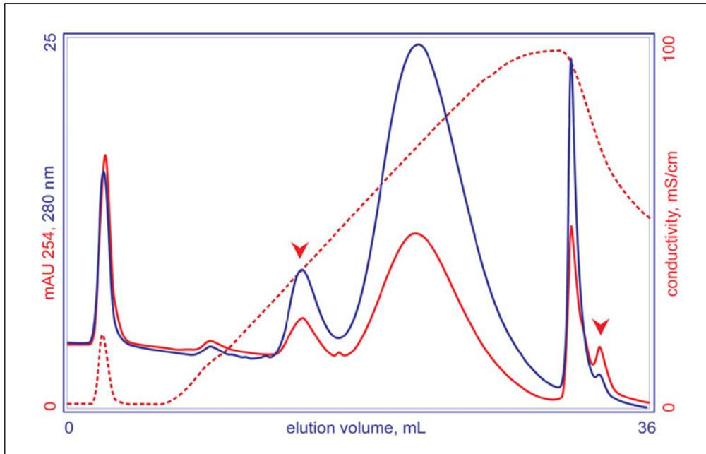
FIGURE 4. HA fractionation of CX-captured IgG in a sodium chloride gradient at 10 mM phosphate, pH 7.0. No secondary wash. Note the super-contaminant and DNA peak (red arrowheads).
