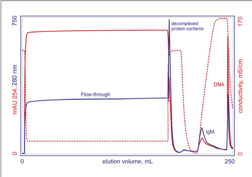
FIGURE 11. IgM capture by HA from cell culture supernatant, eluted with a phosphate/NaCl gradient following a wash with urea and NaCl.
