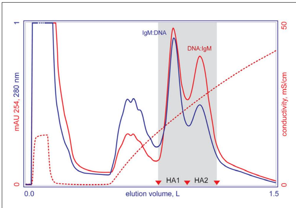
FIGURE 10. IgM capture by HA from cell culture supernatant, eluted with a linear phosphate gradient.
