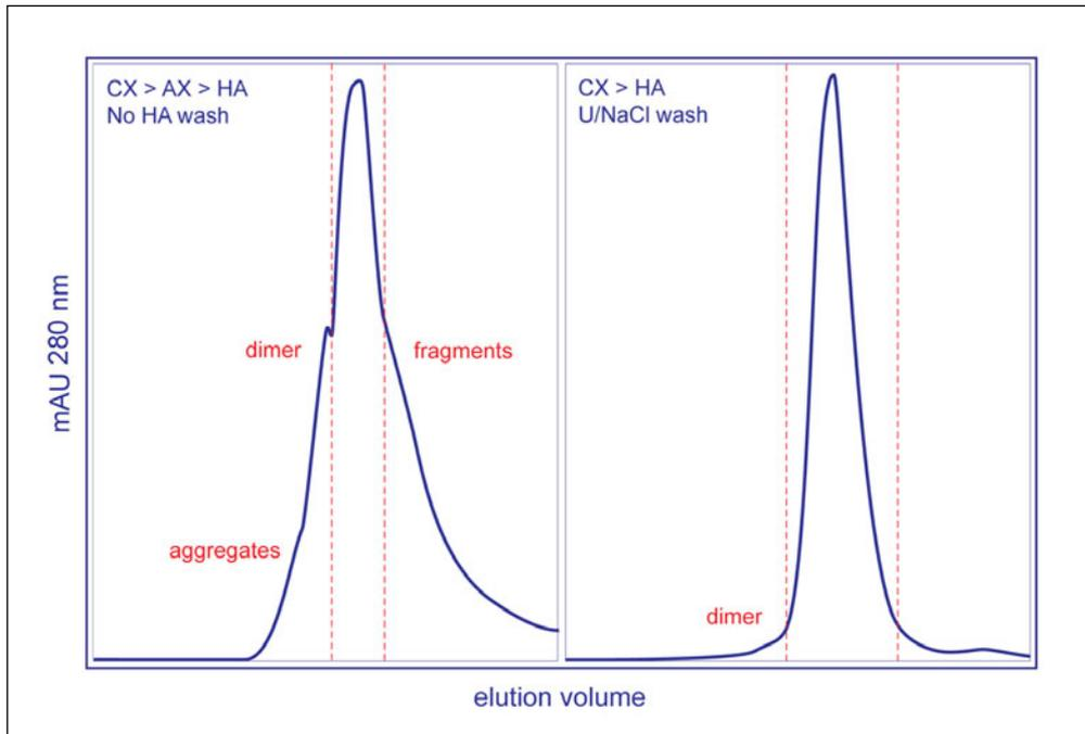
FIGURE 7. Comparison of analytical SEC profiles illustrating the benefits of a secondary wash at the HA step. The first profile shows the results of a three-step purification including HA but lacking a secondary wash. The second profile shows the results of a two-step purification where HA includes a secondary urea/NaCl wash.
