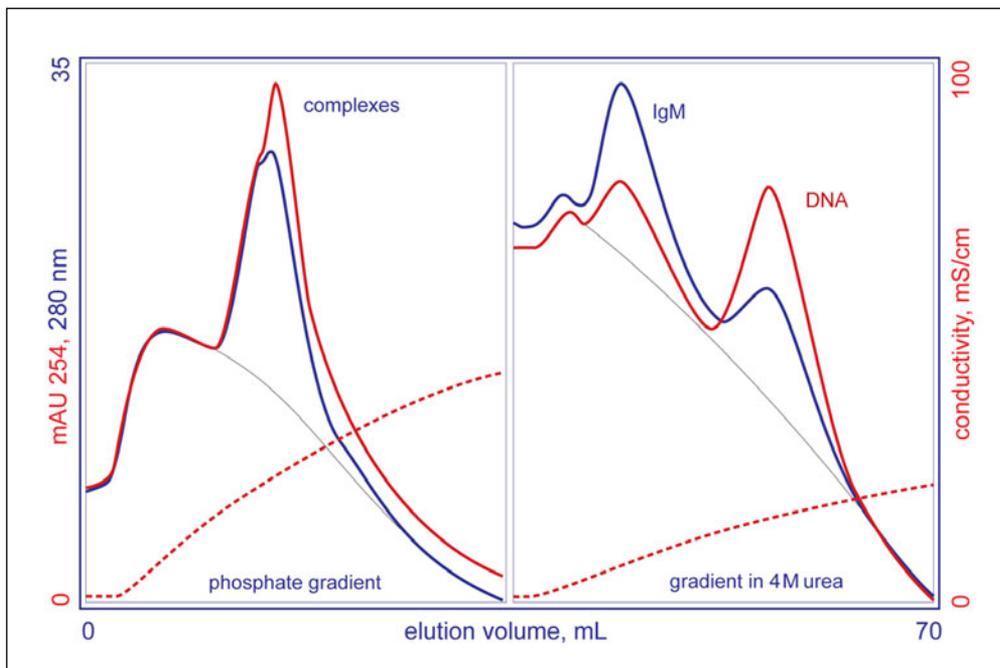
FIGURE 8. Comparison of HA profiles illustrating the ability of urea to promote dissociation of IgM-DNA complexes. The first profile illustrates phosphate gradient elution without urea. The second, level 4 M urea across the gradient. The phosphate gradients are identical. Urea depresses apparent conductivity.
