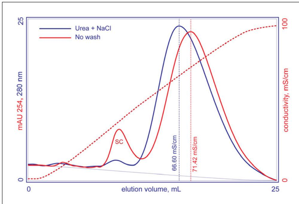
FIGURE 5. Comparison of wash treatments on HA. The red profile is the experimental control (Figure 4) eluted without a secondary wash. The blue profile illustrates elution following a secondary wash with 3.2 M urea and 1.6 M NaCl.
