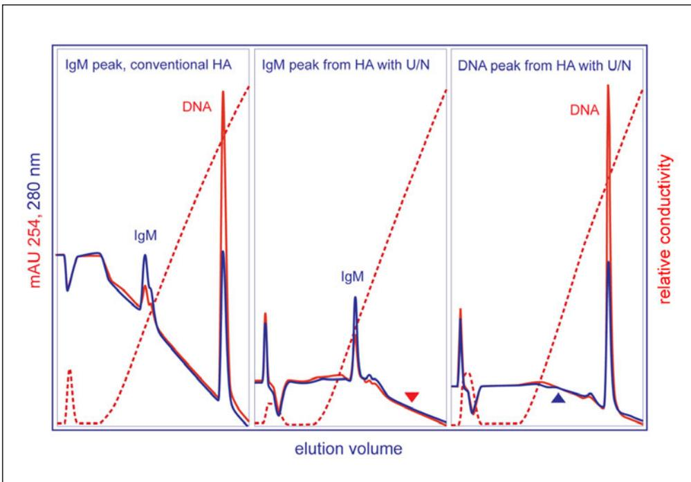
FIGURE 12. Analytical anion exchange on monolithic exchangers. The first profile shows dissociated IgM-DNA complexes from the IgM peak in Figure 10. The second shows the IgM peak from Figure 11, and the third, the DNA peak, also from Figure 11. The red triangle marks the elution point of DNA. The blue triangle marks the elution point of IgM.
