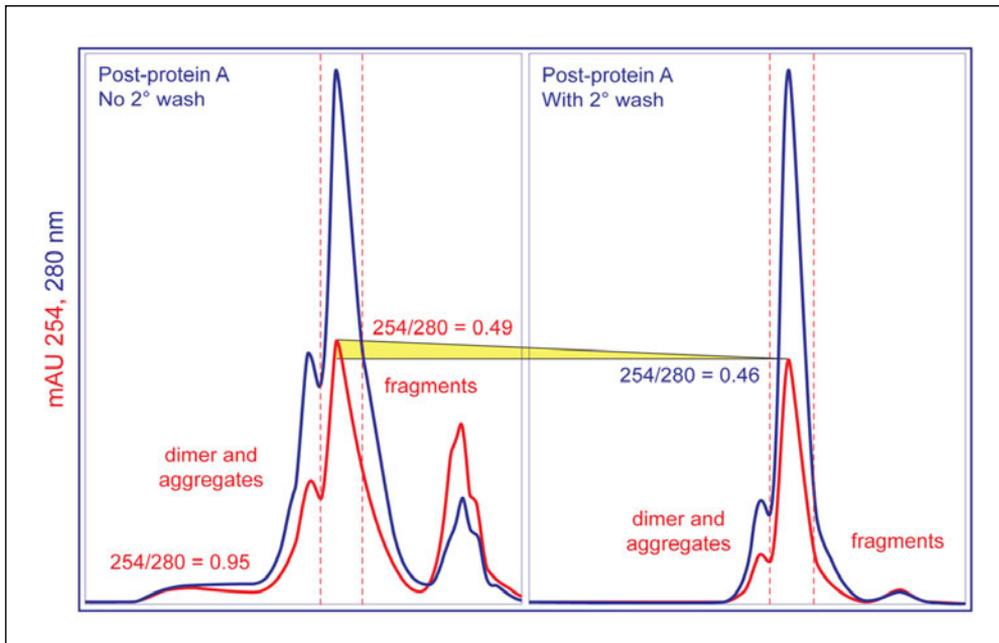
FIGURE 2. Analytical SEC of IgG eluted from protein A affinity chromatography without a secondary wash (first profile), and with a secondary wash (second profile).
