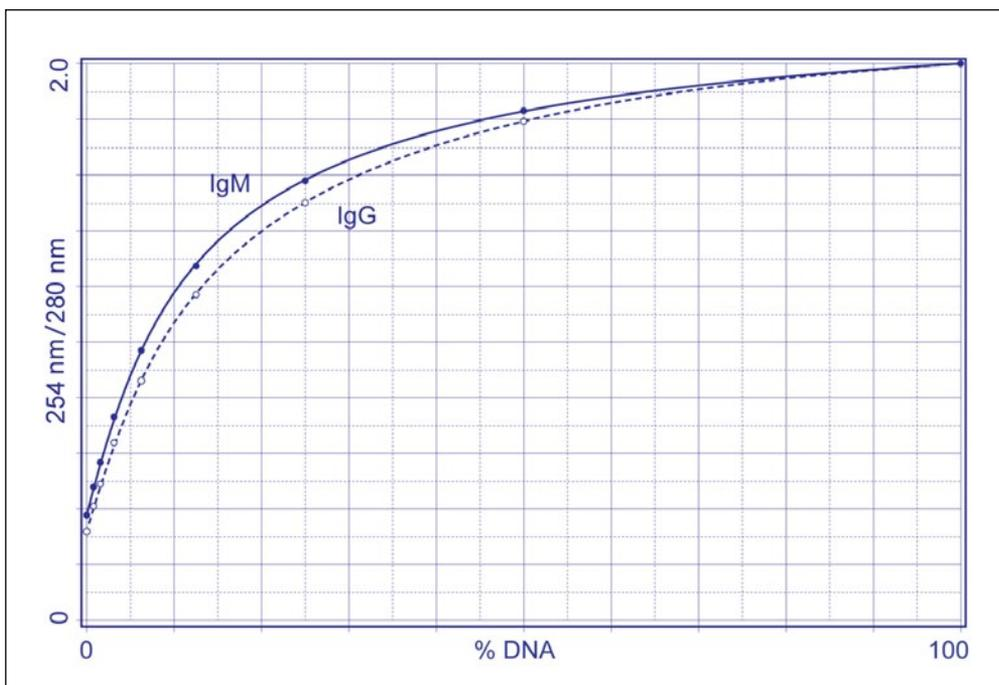
FIGURE 3. Proportioning of DNA versus protein mass according to UV absorbance ratios at 254 and 280 nm. Indicated points were calculated from the equation in Table 1.
