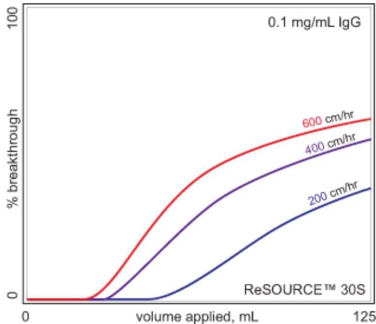
These curves illustrate the process of saturating the binding surface of a column of packed particles (cation exchange). 100% efficiency would be indicated by a vertical line at the point of saturation. Preferential void flow and eddy dispersion contribute to the gradually sloping breakthrough, but the dominating factor is the low efficiency of diffusive mass transport, which manifests as decreasing capacity with increasing flow rate.
