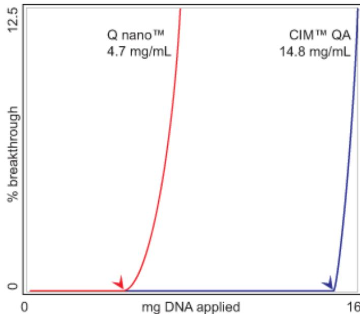
Experimental determination of dynamic binding capacity
