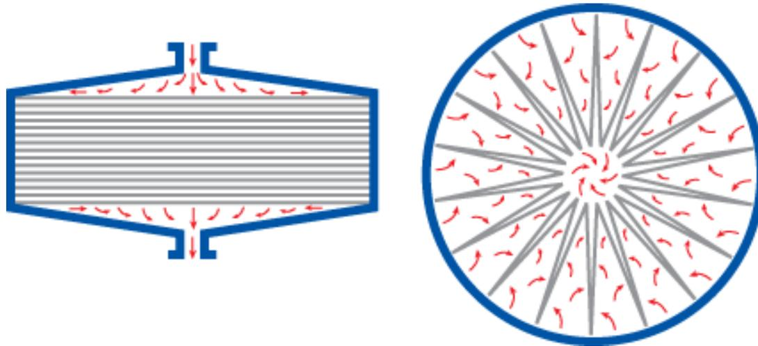
Left: stacked membrane format. Right: pleated cartridge format. These are two of several strategies to increase capacity by putting as much surface area as possible into a fixed volume housing. Some space nevertheless remains unoccupied, where turbulent mixing can occur, and some membrane surface may be poorly accessible.
