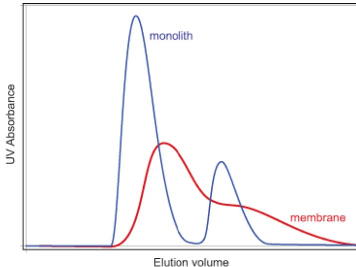
*Internal mixing erodes peak boundaries, reduces resolution, and dilutes the eluted product. Additional steps are required to achieve the desired purification; or it becomes necessary to take narrow fractions and discard the contaminated tails, which reduces product recovery. Increased elution volume increases loading time at the next step.*
