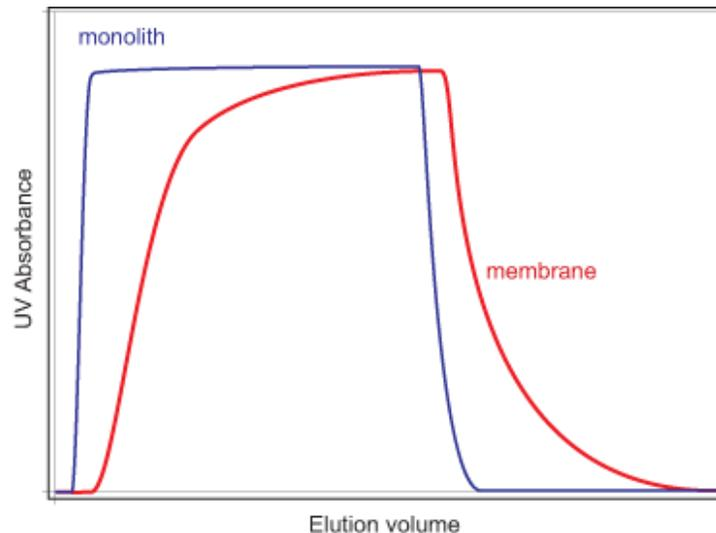
*Internal mixing retards clearance of sample after loading. A prolonged wash is required. Otherwise, product elution may occur while significant contaminant levels are still being applied to the media. This is a particular concern when the objective is to reduce highly regulated contaminant classes to very low levels.*
