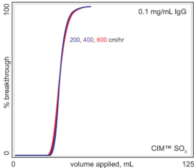
*These curves illustrate the process of saturating the binding surface of a cation exchange monolith.*
