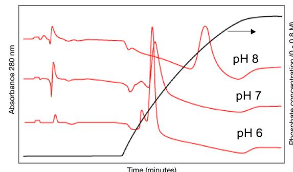
**Figure 2:** Effect of pH on DNA elution from CHT.
